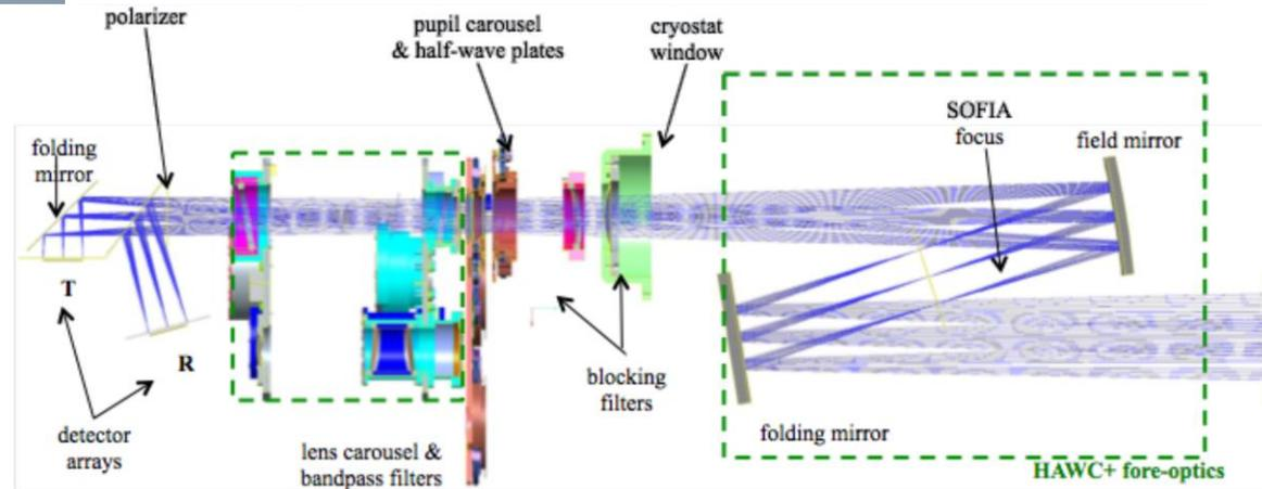
Full Stokes vector can be constructed from four distinct positions of the half-wave plate
